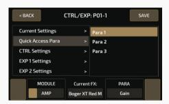
Use MODULE to select the target module. If you don't want the quick access para on, select OFF to turn its function off. When a quick access para is off, the parameter panel will display the status as shown:
