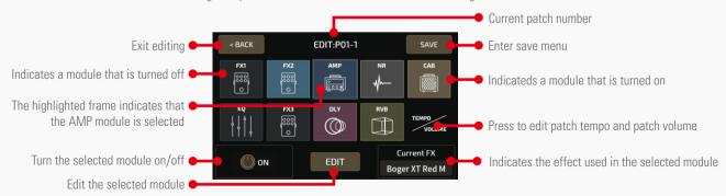
The menu is made of ten icon squares representing Ampero One's nine effects modules and a volume/tempo module. The default signal chain is ordered like this:
