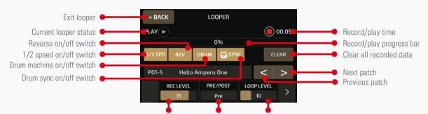
Controls looper recording level Switches looper position Controls looper playback level (pre/post effects)
