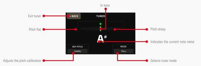
On the upper part is a scale that indicates your pitch. Left of center is flat, and right of center is sharp. As you tune your instrument towards the middle, the color of the scale will change from red (out of tune) to yellow (near pitch) to green (in tune).
