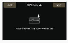
Then press the pedal all the way down and press NEXT.
