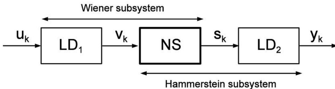
The Wiener-Hammerstein model is composed of the Wiener subsystem and the Hammerstein subsystem. Among them, LD1 and LD2 represent the linear part, which can be simply understood as EQ, which will modify the frequency response of the input signal. NS represents the non-linear part. It is understood as a non-linear device (such as a diode or a vacuum tube), which will change the shape of the input signal waveform, resulting in clipping distortion.
