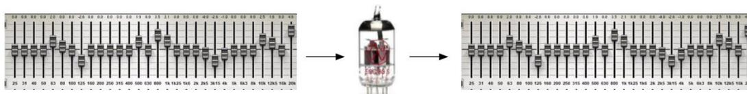
The Wiener-Hammerstein model can be widely used because it is able to easily and efficiently represent the module functions of most distorted circuits (although it cannot represent its circuit topology).
