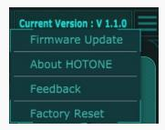
Then click "Update Firmware" button on the bottom, choose the firmware file location, and click "OK". The Binary pedal cannot be operated until the update process is complete.
